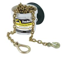
GRADE 70 LASHINGS & FITTINGS ARE NOT TO BE USED FOR LIFTING PURPOSES \* NOTE: The use of some grab hooks or systems incorporating grab hooks cause bending to occur on the link of lashing chain to which the grab hook is engaged. The bending and shearing effect of the hook reduces the strength of the chain by 25 percent and as such, the lashing capacity (LC) of this type of system must be reduced by 25 percent as prescribed in Australian Standard AS/NZS 4344
